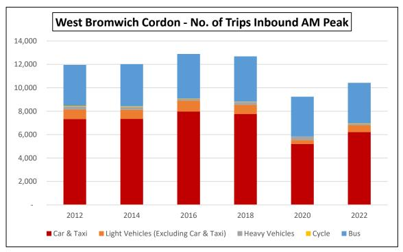
The AM Peak (07.30-09.30) public transport mode share has decreased slightly in 2022 to 40.0% (bus 35.3%, tram 4.7%) from 40.4% in 2020, mainly due to an increased in trips using private vehicle modes (except heavy vehicles) and a decrease in tram trips.
